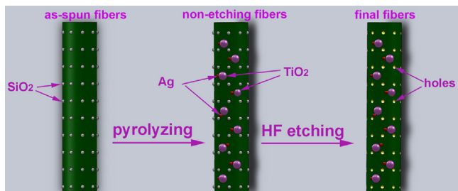
Fig. 6. The schematic diagram represents the formation mechanism of PNATC.
