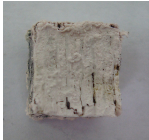
Fig. 9. The composite sample after the acetylene flame test for 10 min.
