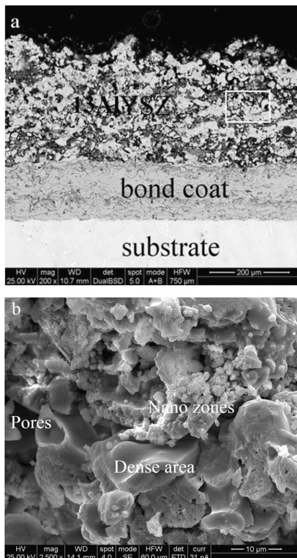
Fig. 2. Cross section (a) and the fractured cross section (b) of nano-13AlIYSZ coating.
