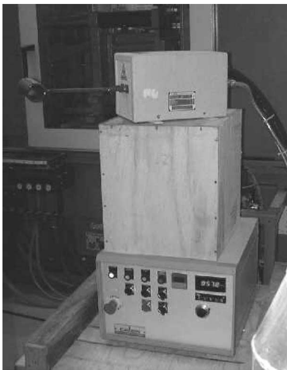
Fig. 3. Induction melting device provided by Celes (Lautenbach, France).
