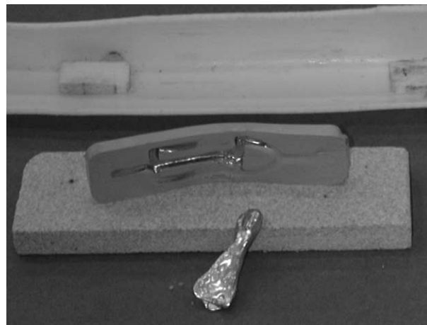
Fig. 6. Removal of the core by induction melting from a sample moulded with EVA-2 binder.
