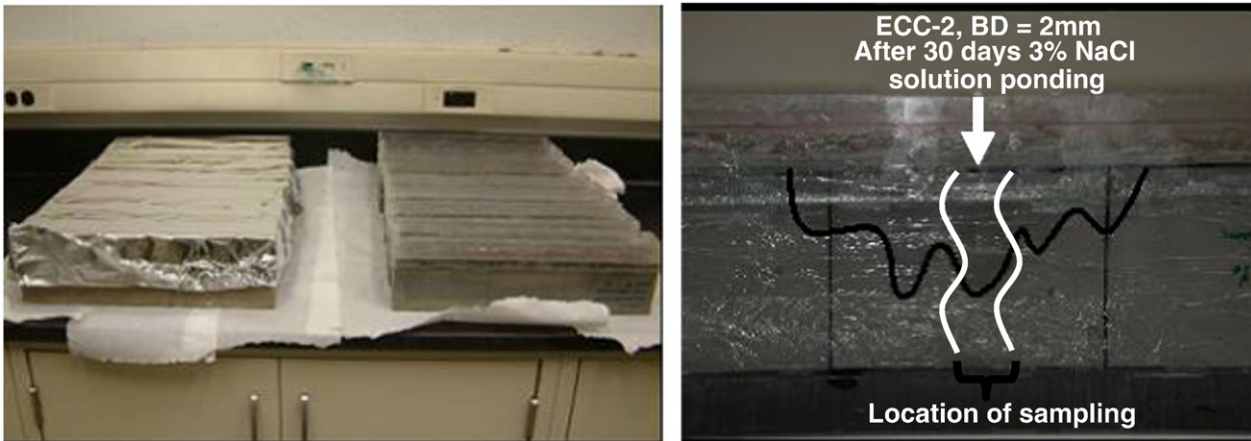
Fig. 3. Typical ECC prisms (355×75×50 mm) during and after 30 days salt solution exposure and location of the sampling for chloride profiling.
