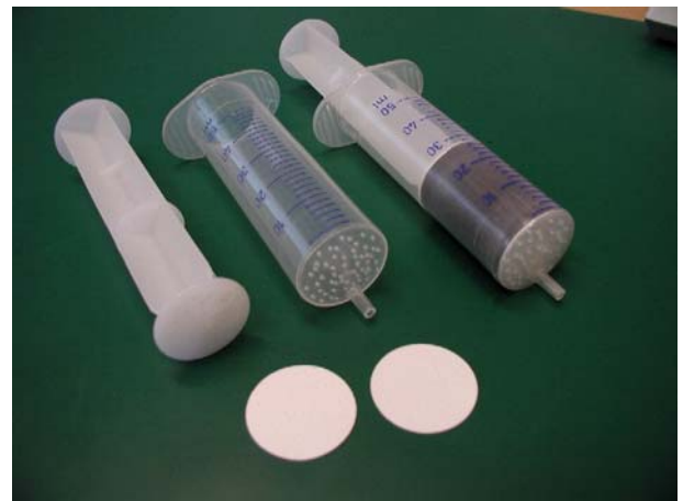
Fig. 1. Equipment used for packing experiments, one unused syringe is shown in a dismantled state the other syringe shown has been used for a packing experiment.
