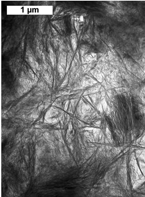
Fig. 14. A TEM micrograph from the KOH-activated paste hydrated for 28 days showing foil and lath-like Op C–S–H.
