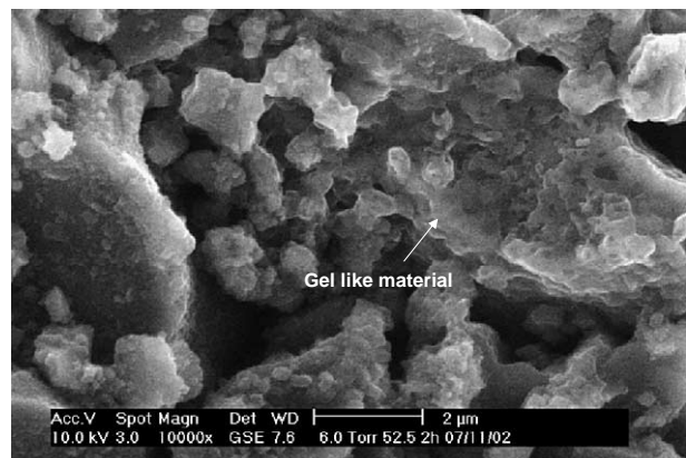
Fig. 8. ESEM micrograph of P (0% admixture) after 2 h of curing.
