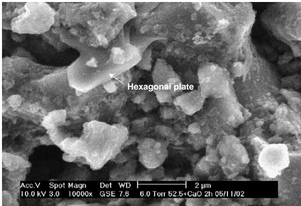
Fig. 9. ESEM micrograph of P (3% EXP) after 2 h of curing.
