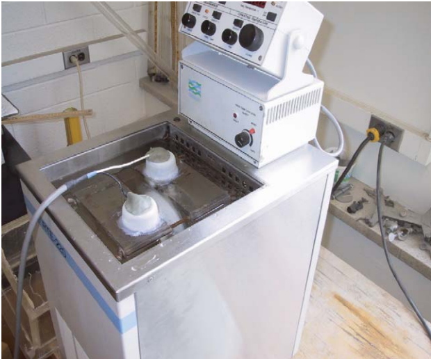
Fig. 1. Test arrangement (water bath and RCPT cell).
