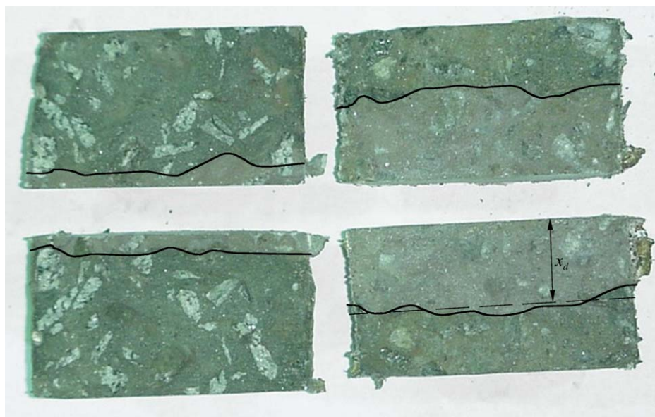
Fig. 10. Measurement of chloride penetration depth.
