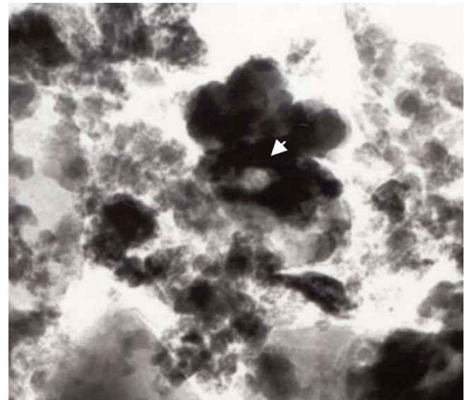
Fig. 5a. Bright field of the SCBA1, enriched in Ca.
